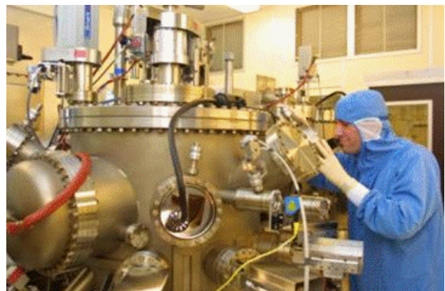
Gas-source MBE for QD epi-wafers fabrication (III-V Lab)
