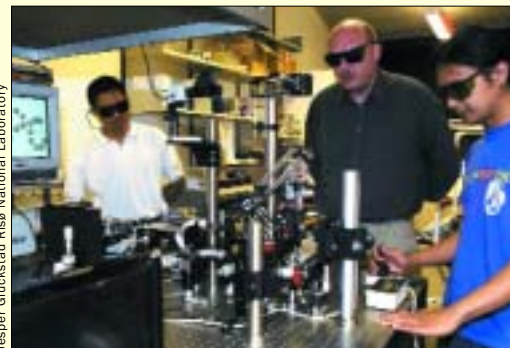
Optical tweezers developed at Risø National Laboratory for 3D real-time manipulation of small particles are an example of Denmark's strength in photonics.
