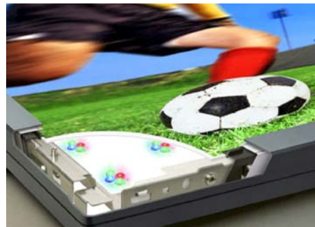
In this detail of the OSRAM flat-panel display, the corner has been cut away to reveal the placement of the backlighting LED clusters underneath.
