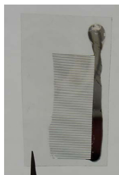
Figure 1. (top) Cell exploiting the Ag grid. (lower left) Ag grid on plastic sheet. (lower right) Current-voltage characteristics from three cells exploiting electrodes based on PEDOT(PSS). The three electrodes compared include one pure DEG-PEDOT(PSS), one (ITO)+PEDOT(PSS), and one exploiting Ag grid+DEG-PEDOT(PSS). PEDOT(PSS): Poly(3,4-ethylenedioxythiophene) poly(styrenesulfonate). DEG: Diethylene glycol. ITO: Indium tin oxide.
